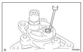
26. REMOVE TRANSFER OIL PUMP BODY O-RING
