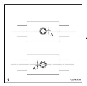
(g) Using a pin punch and hammer, install the slotted pin.
